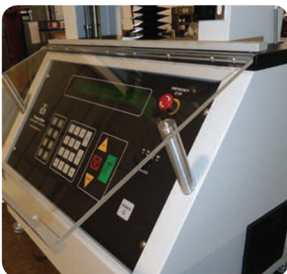
▲ QC-3A Splash Guard (Part No. 1476-0080) is recommended for use with wet samples to keep the keypad protected.
