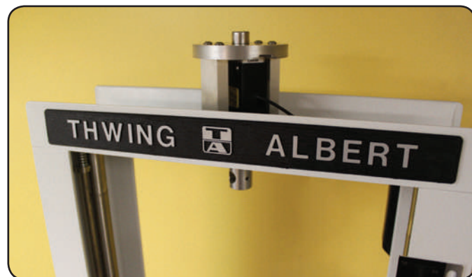
▲ QC-3A Load Cell Adapter (Part No. 771-3000) can be ordered to move the load cell outside of the frame to add extra crosshead travel.
